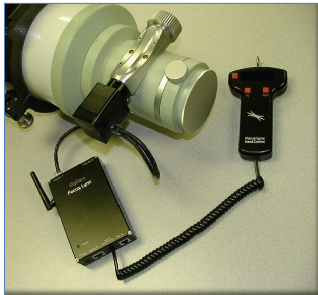
FocusLynx Controller Hub configured for MicroTouch motor. (Shown with FeatherTouch MPA/TRF pinion assembly on Takahashi TOA-130)
