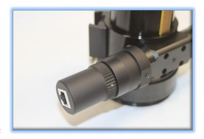
Developed as an improvement over the original QuickSync SV motor, DirectSync SV provides a direct geared connection to the focuser rack and pinion assembly. The system will not slip and can carry loads in excess of 5 kg (11 lbs.) with excellent repeatability. The DirectSync SV uses a clutch mechanism and a simple twist of the motor housing disengages and re-engages the motor.
