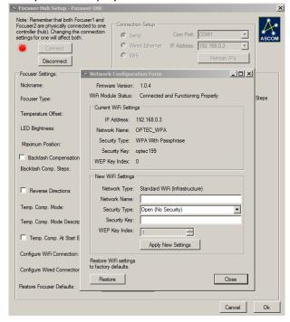
Once the FocusLynx WiFi receives a valid IP address from the local WiFi router, you may disconnect the Serial connection, click the WiFi radio button and click the "Refresh IP's" button. Allow at least 30 seconds for the local PC to find the FocusLynx WiFi board on the network. Click Connect and you will be able to control the FocusLynx hub using FocusLynx Commander and the ASCOM drivers.
