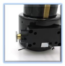
Adjust the gear position so the hub setscrew can be tightened. Insert the 1/16" hex key into the access port to tighten the gear to the pinion shaft. Be sure it is fully secured before continuing.
